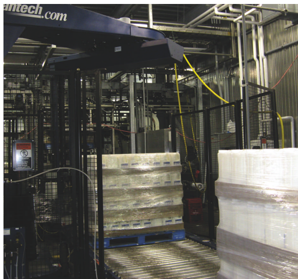
The unique bottle design allows a four-high stack to contain more gallon bottles than the six-high stack with the usual bottle design. After palletizing, the pallets are stretch-wrapped for shipment.
