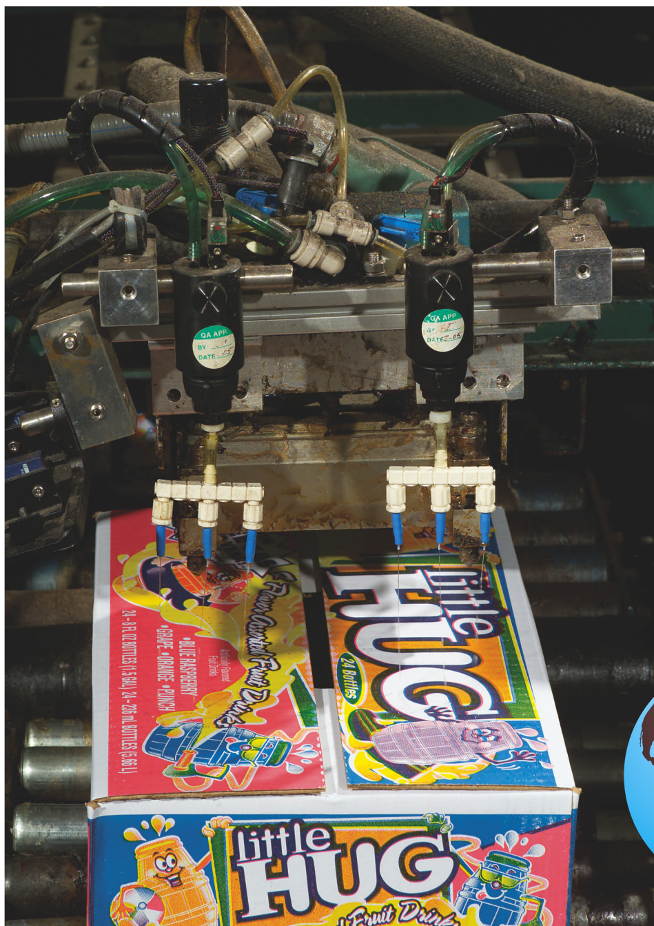
Easy-release adhesive is sprayed from nozzles onto the cases of juice, above, at Daily's Verona, PA, facility. An air-driven pump connected to a drum of adhesive, right, supplies the nozzles with the adhesive, which is used to unitize pallet loads before stretch wrapping.
